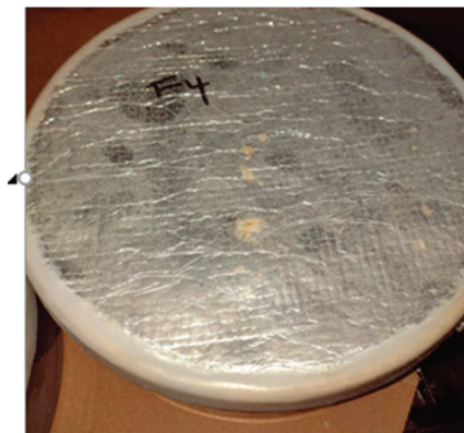
Figure 4. Mould growth on specimen E.
