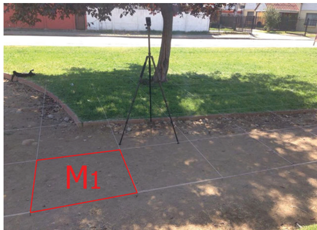
Figure 4. Location of the spectrometer in a quadrant to take the measurements.
