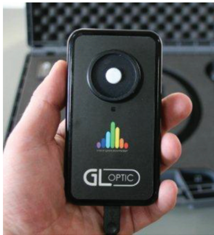
Figure 1. GL optic mini-spectrometer.
