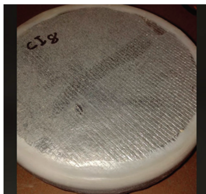
Figure 3. Mould formation on specimen D.
