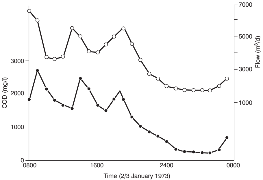
Figure 7.1 Diurnal Variation of Wastewater Flow (○) and Load (●) at Nakuru, Kenya
