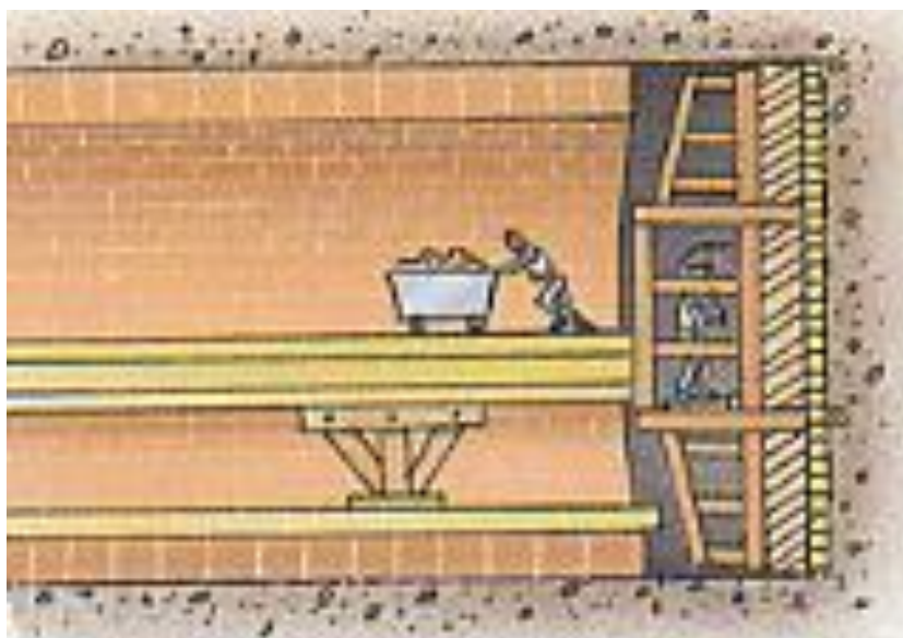
Figure 9.1 – M. Brunel's tunneling shield
