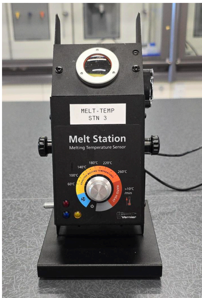
Figure 12. The Vernier Melt Station (sometimes referred to as a “meltemp”). The figure was created by Gustavo Casanova, CC BY-NC.
