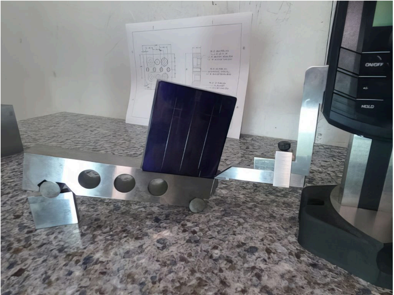
Figure 14-7. The sine bar is used to scribe an angular line accurately.
