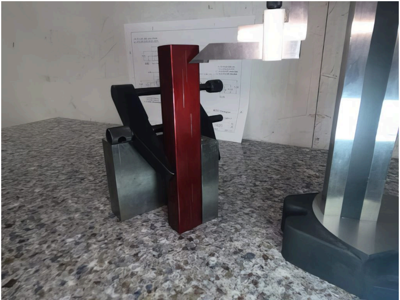
Figure 14-4. An angle plate is used to secure the part for a vertical layout.
