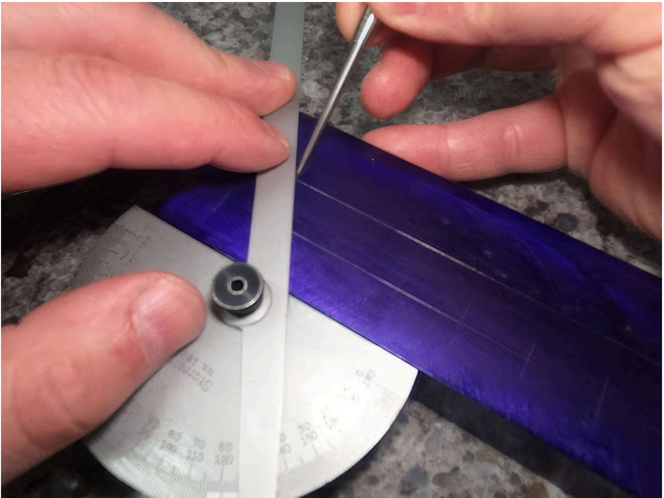
Figure 14-6. A protractor is used to scribe an angular line on a part.
