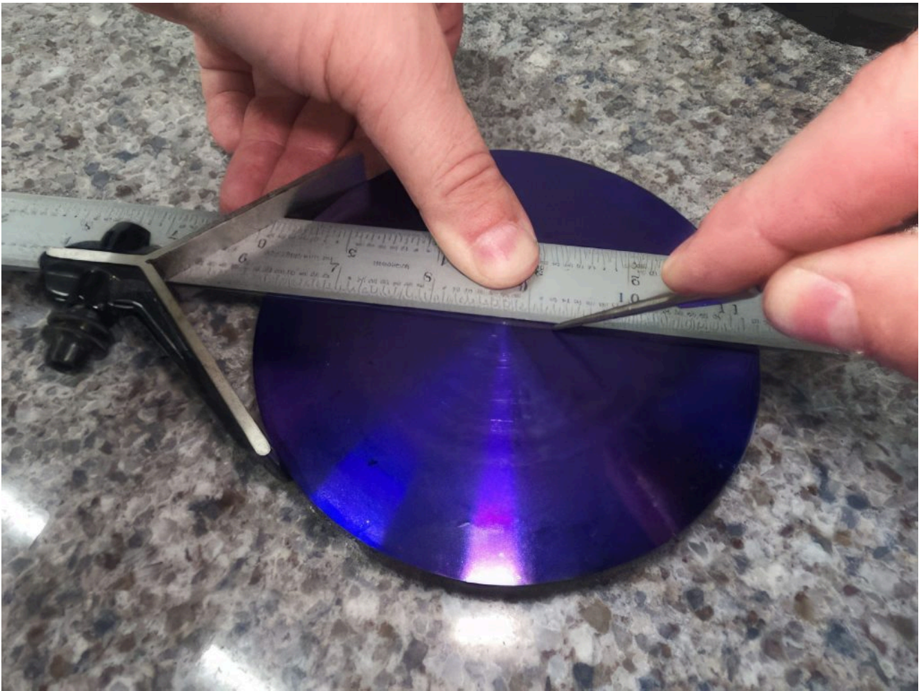
Figure 14-2. A scribe is used to create an accurate line on a part of the surface.
