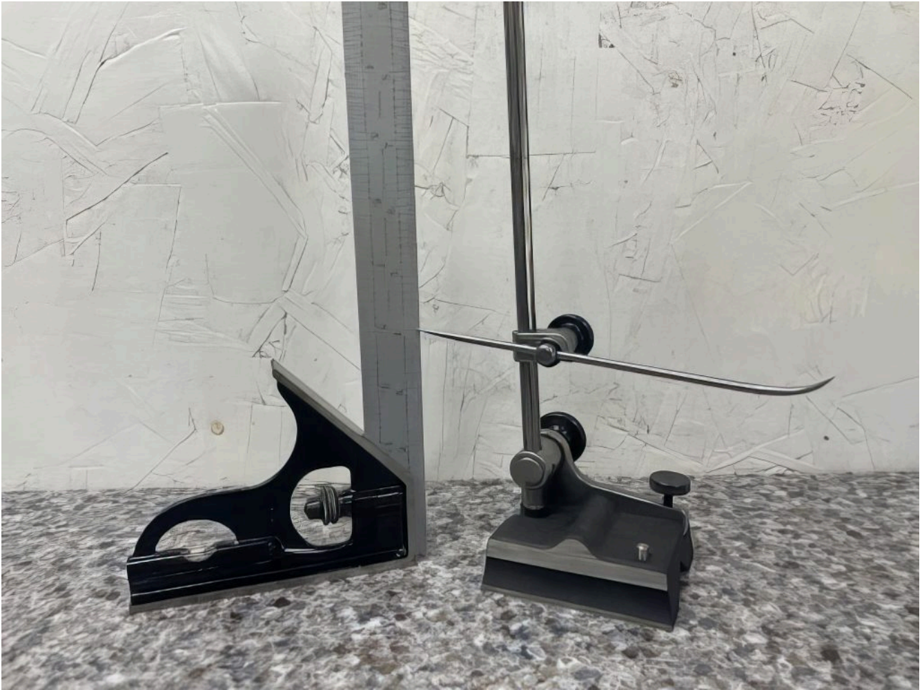
Figure 14-5. The surface gauge is set to a height measurement for scribing.
