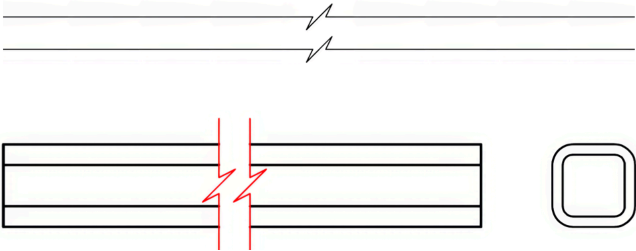
Figure 3-14. Long break line allows the removal of a portion of a longer part to shorten a drawing view.
