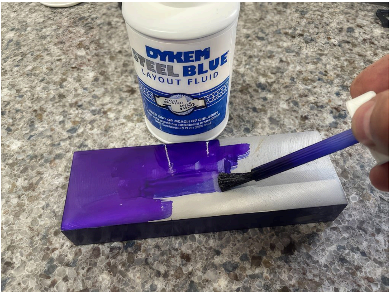
Figure 14-1. Layout fluid applied to a part surface.
