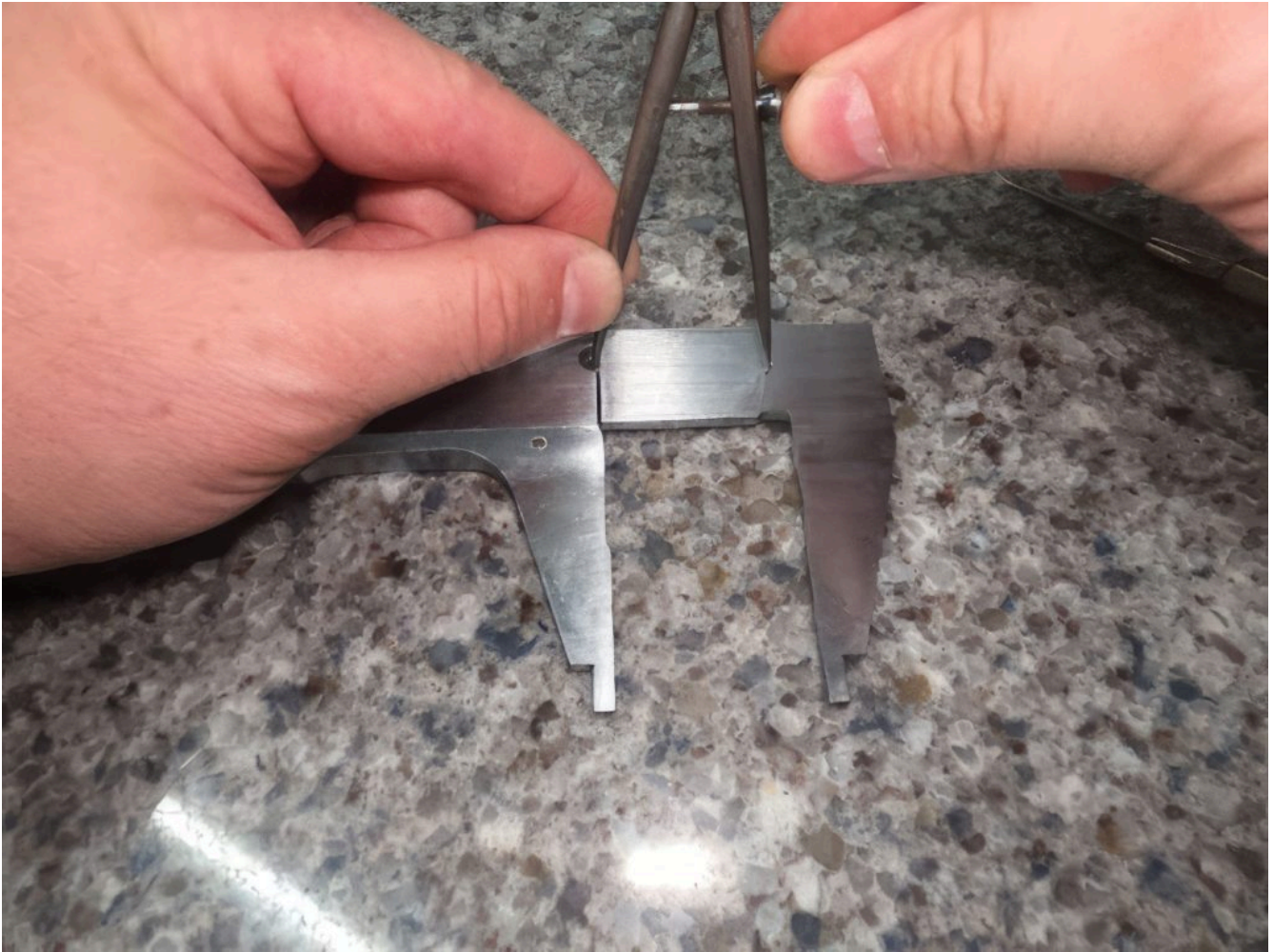
Figure 14-9. A divider is set using indents on a caliper.
