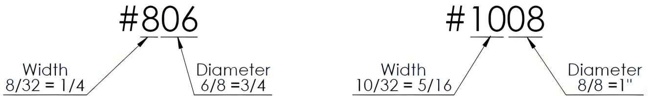
Figure 10-11. A Woodruff key is identified by the width in 32nds of an inch and diameter in 8ths of an inch.
