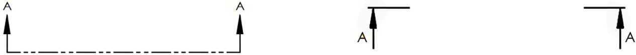
Figure 3-6. Additional line styles may be used for both cutting-plane and viewing-plane lines.
