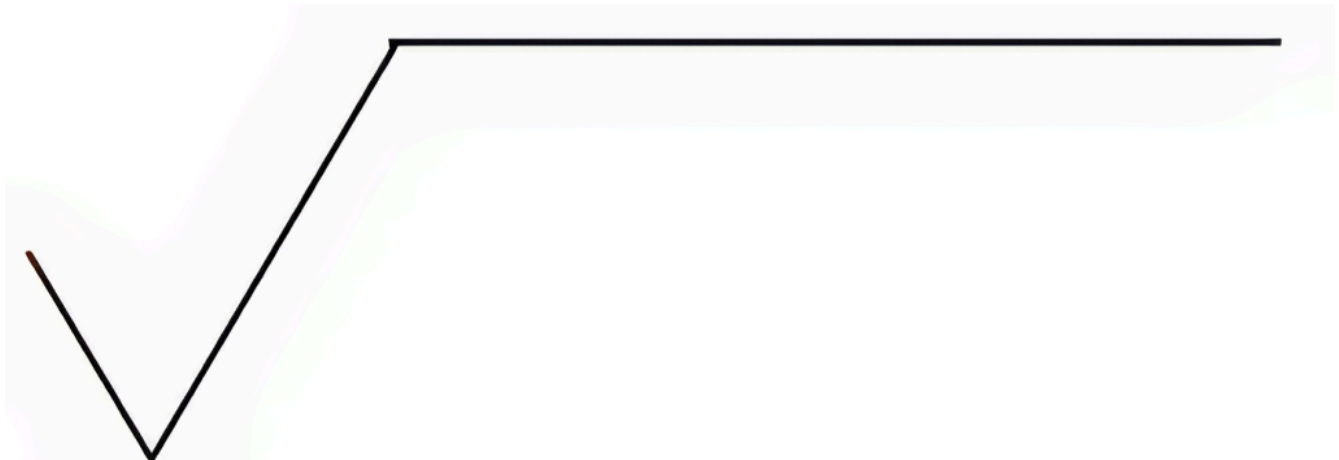
Figure 9-16. A surface texture symbol with a horizontal line is used to provide additional surface information.
