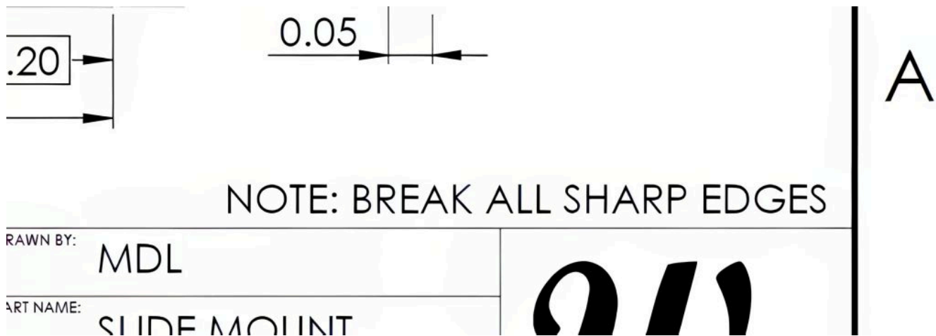
Figure 9.1. General note applies to the entire drawing and is often placed near the title block.
