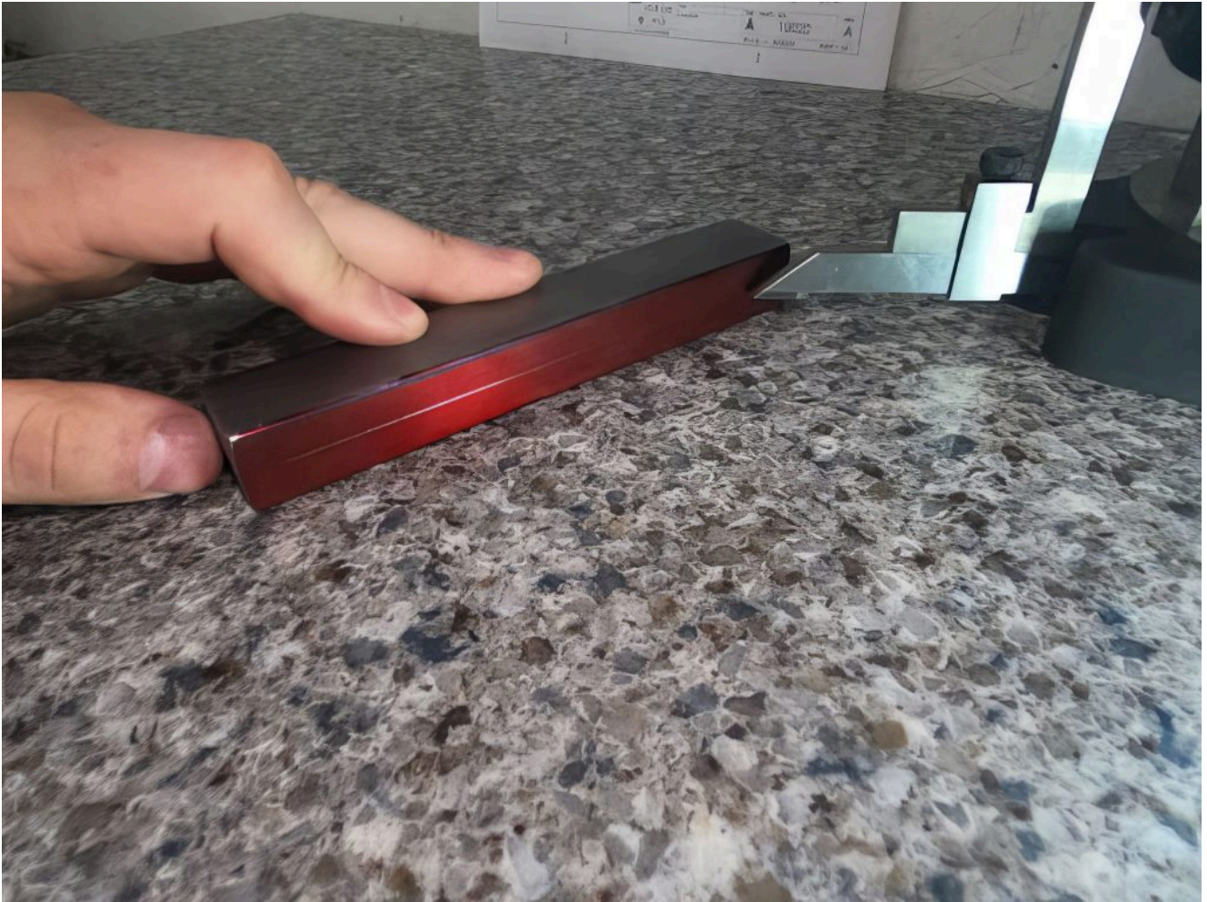
Figure 14-3. A scribe line was created using a surface plate and height gauge.
