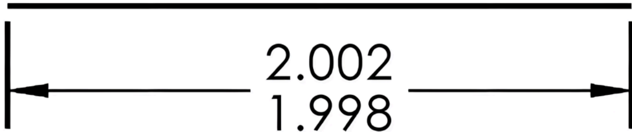
Figure 8-4. Limit dimension – the size for this dimension may range between 2.002 and 1.998.
