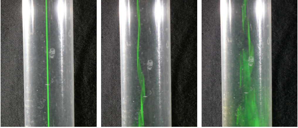
Figure 6.1: A replica of Reynolds’ dye experiment for exemplifying the laminar (left) and the turbulent flow (right). The transition between laminar and turbulent is shown in the centre.
