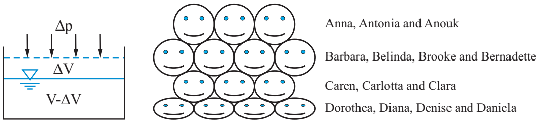
Figure 3.5: Compression of a fluid volume (left) and explanation of the pressure distribution with compressible media (right).
