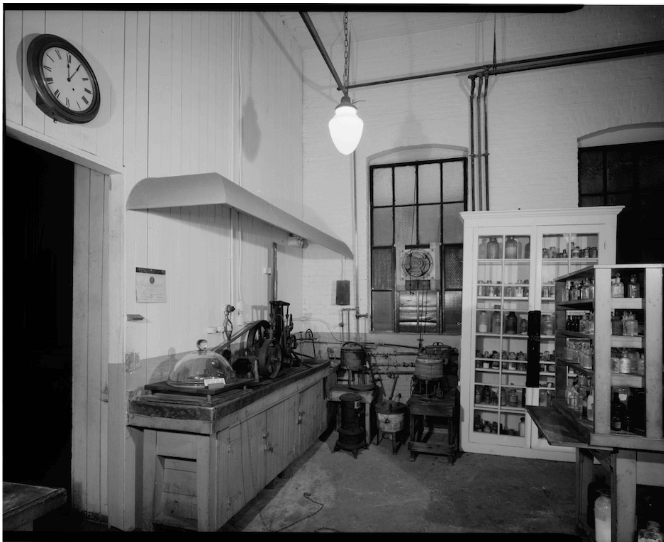
Figure 3. Interior of Thomas. A. Edison Laboratories, Building No. 2, West Orange, New Jersey. Apparatus on the table was used to make a steel master for the mass production of phonograph records. Photo: Jet Lowe, Library of Congress Prints and Photographs Division, HAER NJ,7-ORAW,4-A.
