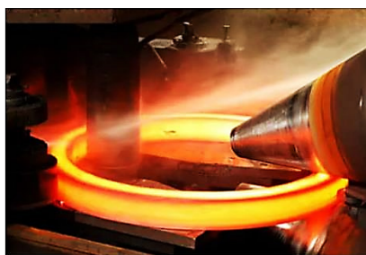
Ring Rolling from a manufacturing plant
