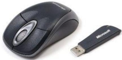
enable the user to control the movement of the cursor on a screen display. Most mice have two or more buttons which allow the user to scroll and click objects on the screen.
