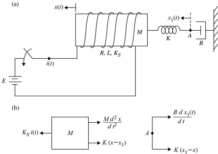
**Fig. 1.63** a Electromechanical system for Example 1.61. b Free body diagram for Example 1.61
