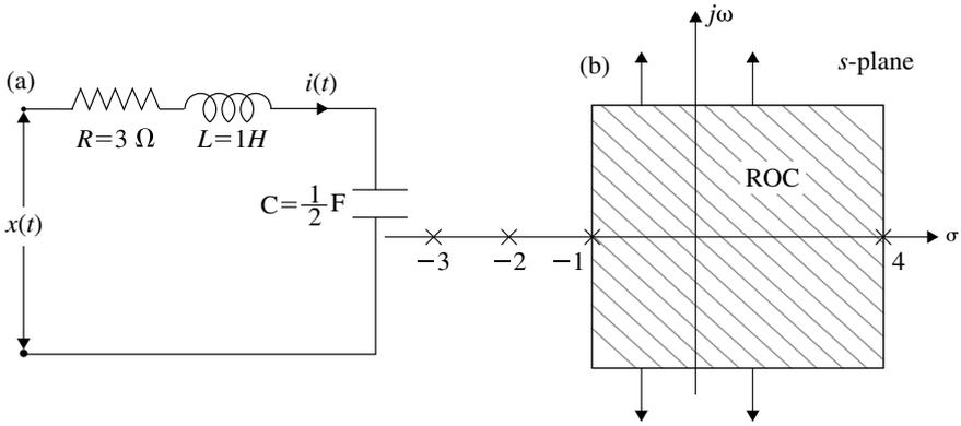
Fig. 4.48 a R.L.C circuit; b ROC of Example 4.89
