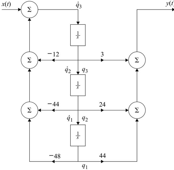
**Fig. 6.12** Direct form-II realization of  $H(s) = \frac{3s^2 + 24s + 44}{(s^3 + 12s^2 + 44s + 48)}$
