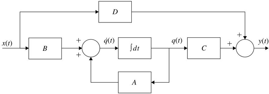
**Fig. 6.1** Block diagram representation of state Eqs. (6.1) and (6.2)
