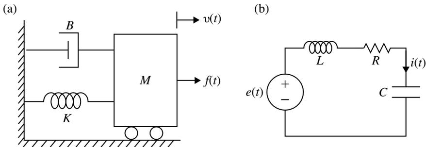
Fig. 1.65 Force–voltage analogy of mechanical system
