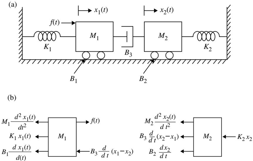
**Fig. 1.61** a Mechanical system for Example 1.59. b Free body diagram for Example 1.59
