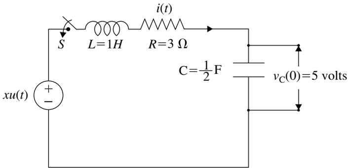
Fig. 4.33 R.L.C. series circuit with initial conditions
