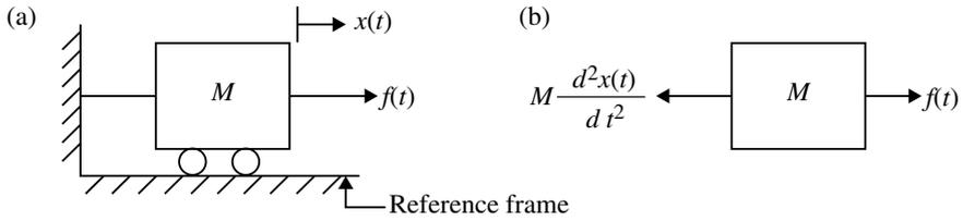
Fig. 1.57 Mechanical system with mass  $M$
