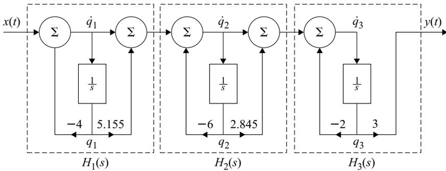
**Fig. 6.13** The cascade realization of  $H(s) = \frac{3(s + 5.155)(s + 2.845)}{(s + 4)(s + 6)(s + 2)}$
