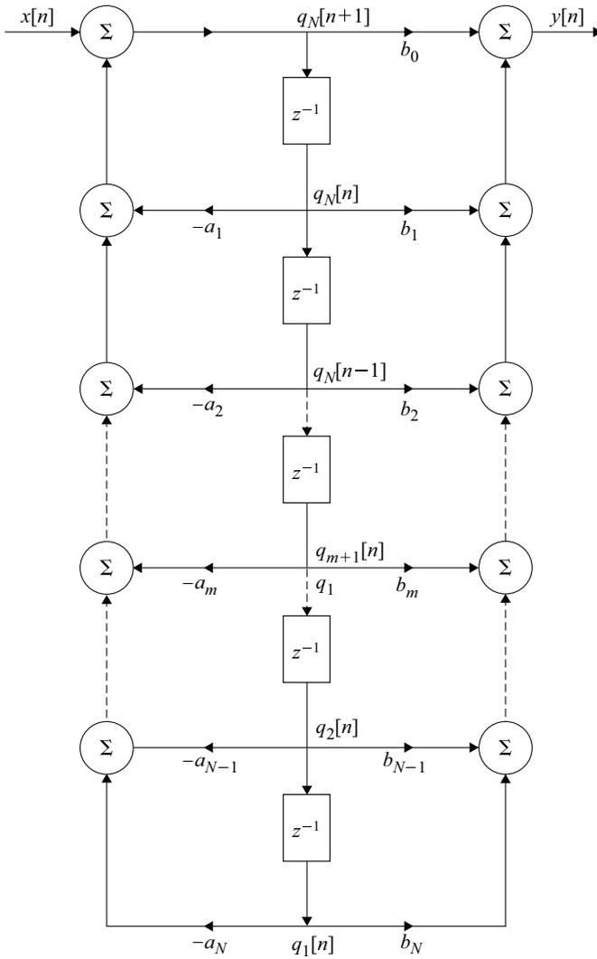
**Fig. 6.17** Direct form II realization of  $N$ th-order discrete-time system
