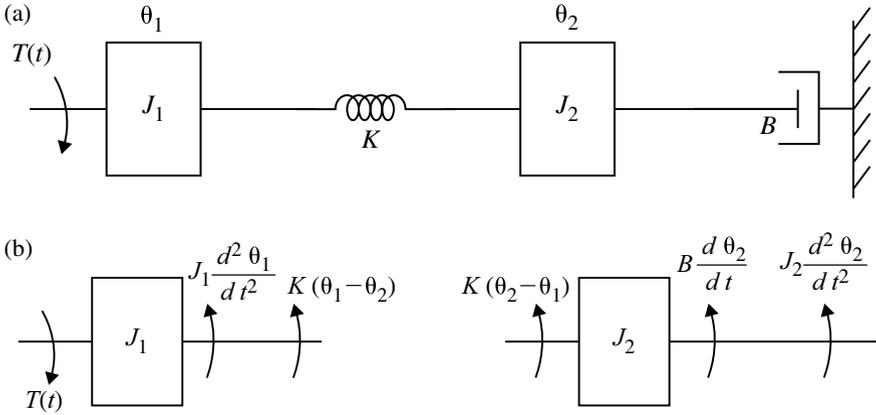
**Fig. 1.64** a Mechanical Rotational System. b Free body diagram for Example 1.62
