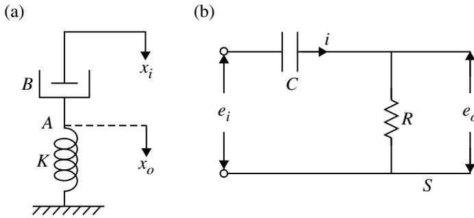
**Fig. 1.69** Mechanical system and electric circuit for Example 1.65
