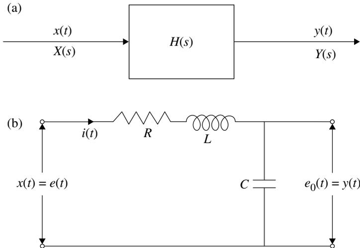
**Fig. 1.50** a Block diagram of CT system. b  $R$ - $L$ - $C$  series electric circuit
