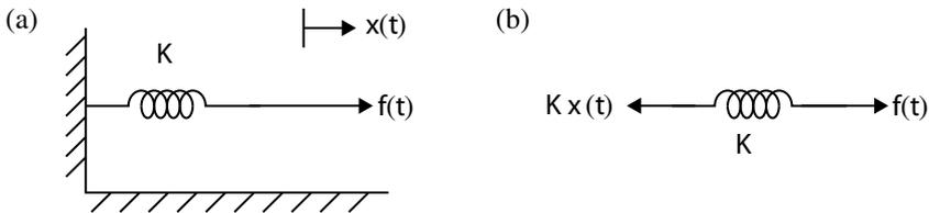
Fig. 1.58 Free body diagram of a spring
