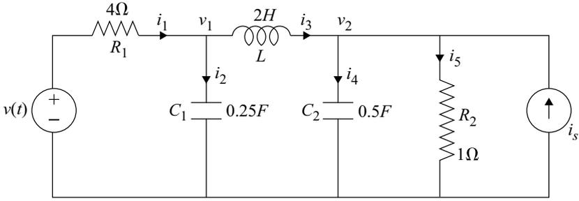
**Fig. 6.8** Electrical network of Example 6.7
