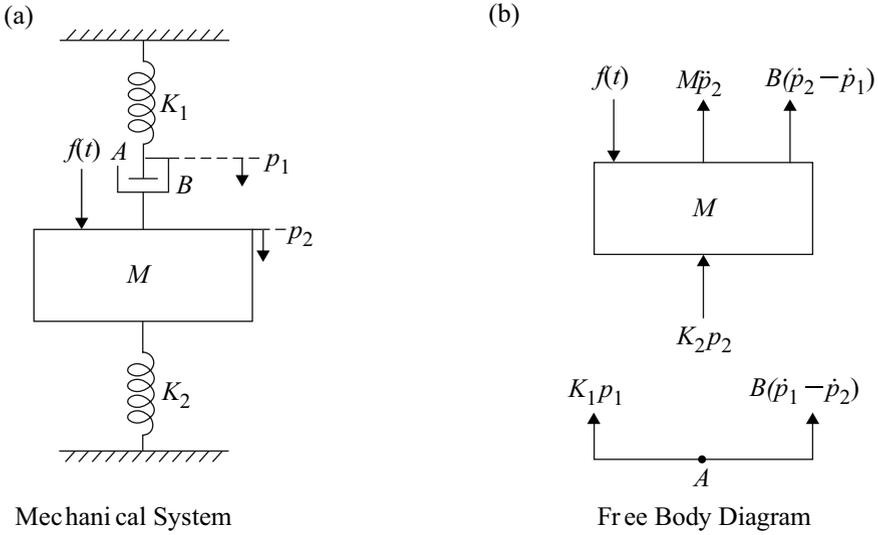
Fig. 6.3 Mechanical system and its free body diagram
