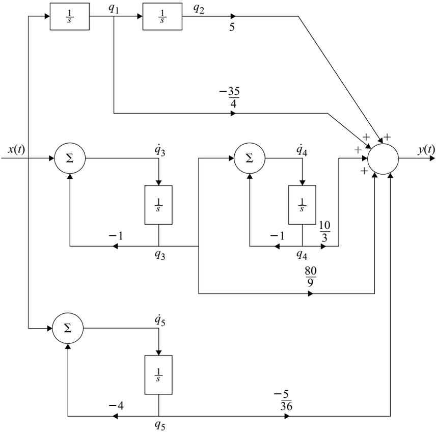
Fig. 6.15 The parallel form realization of  $H(s)$  for Example 6.11
