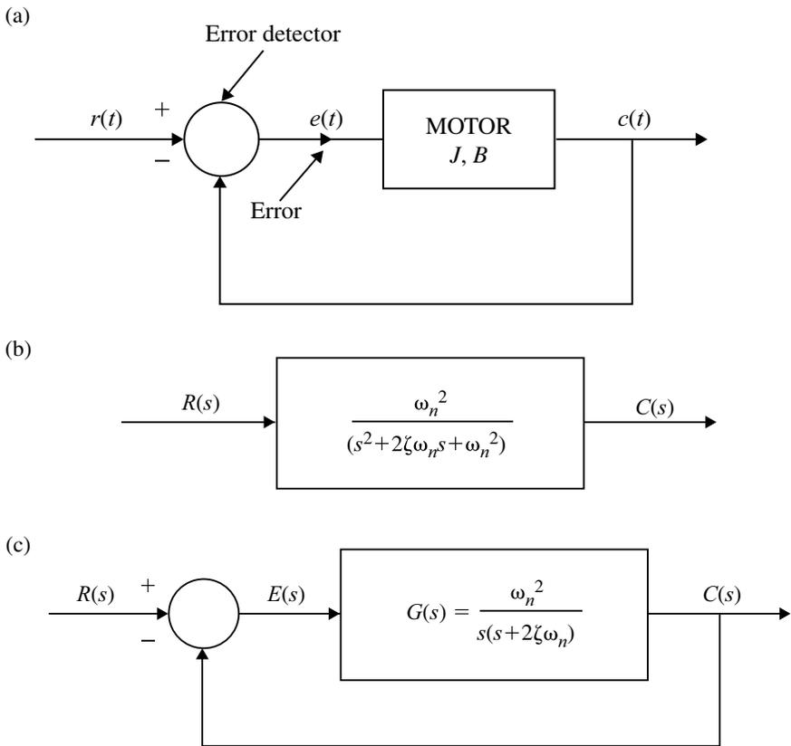
**Fig. 1.74** **a** Block diagram representation of a second-order systems. Second-order system representation. **b** open-loop form, **c** closed-loop form
