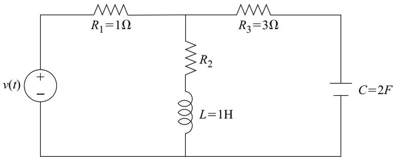
Fig. 6.22 Electrical circuit for Example 6.2
