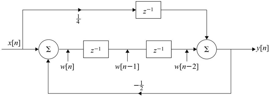
**Fig. 5.18** Block diagram of Example 5.44
