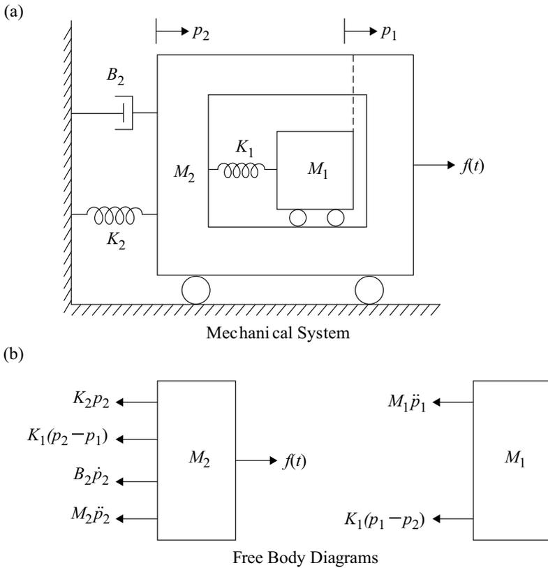
Fig. 6.4 Mechanical system and its free body diagrams
