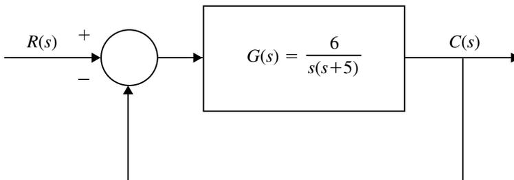
**Fig. 1.83** System block diagram for Example 1.70
