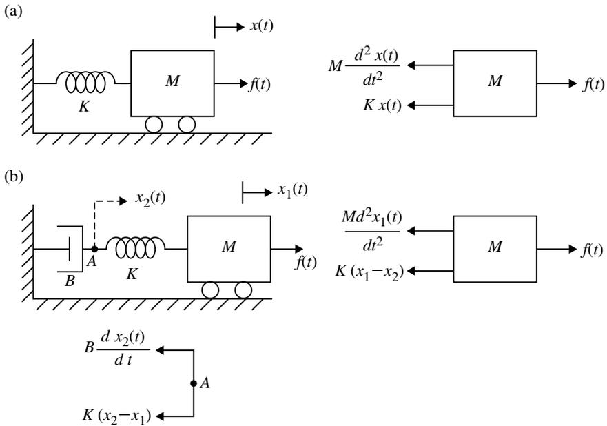
**Fig. 1.60** a Mechanical system component spring connected to the reference frame; b Spring not connected to the reference frame
