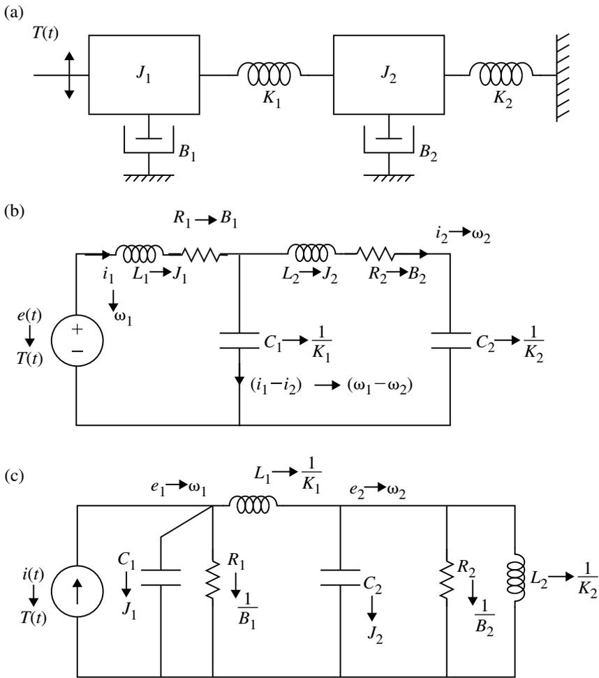
Fig. 1.67 a Mechanical notational system. b and c Electrical analogous circuit for Example 1.63
