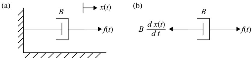
Fig. 1.59 Free body diagram of a dash-pot
