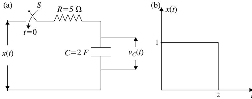
Fig. 4.36 a R.C. circuit and b  $x(t) = u(t) - u(t - 2)$
