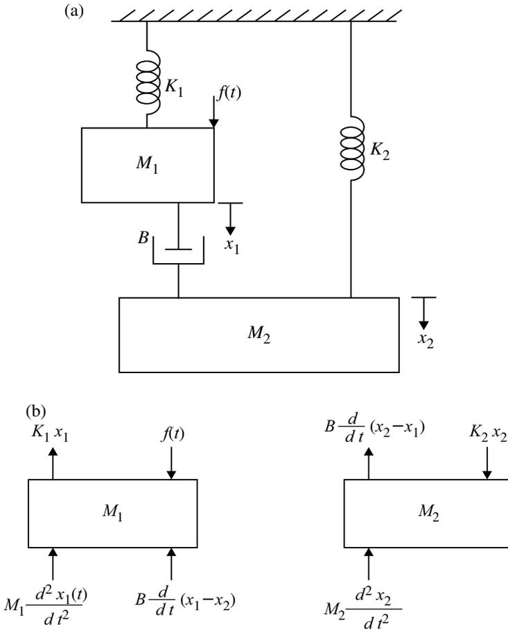
**Fig. 1.62** a Mechanical system for Example 1.60. b Free body diagram for Example 1.60
