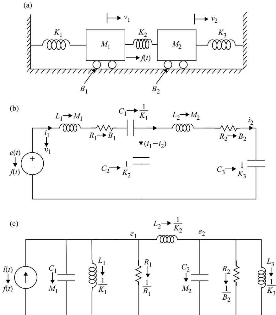
**Fig. 1.93** a Mechanical translational system. b F-V analogous circuit. c F-I analogous circuit
