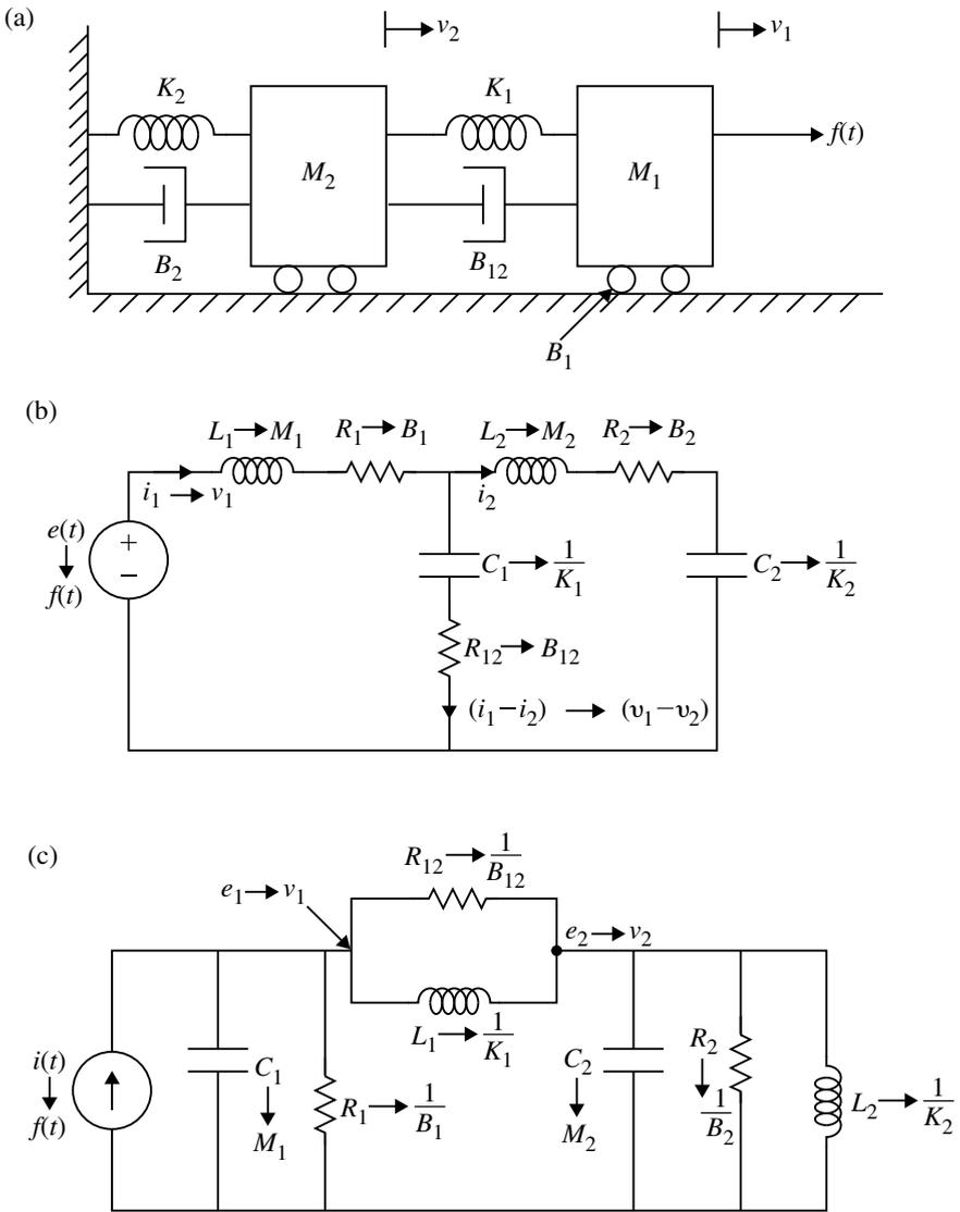
**Fig. 1.68** a Electrical analogous circuits for Example 1.64. b F-V analogy. c F-I analogy
