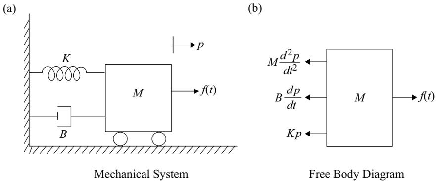
**Fig. 6.2** Mechanical system and its free body diagram
