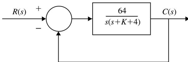
Fig. 1.85 Reduced block diagram of Fig. 1.84
