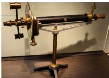
A polarimeter is used to measure optical rotation. By Jerónimo Roure Pérez, CC BY-SA 4.0, https://commons.wikimedia.org/w/index.php?curid=59616417
