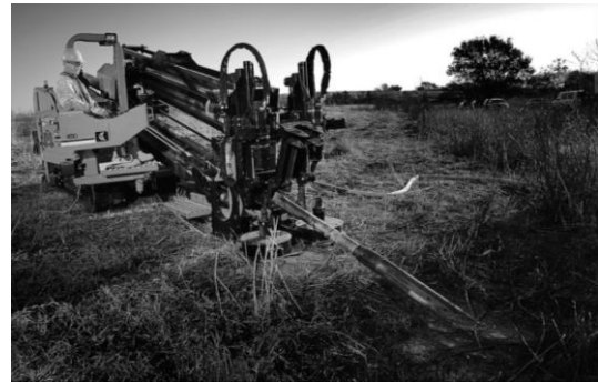
Figure 4.20 Horizontal flush drilling.
