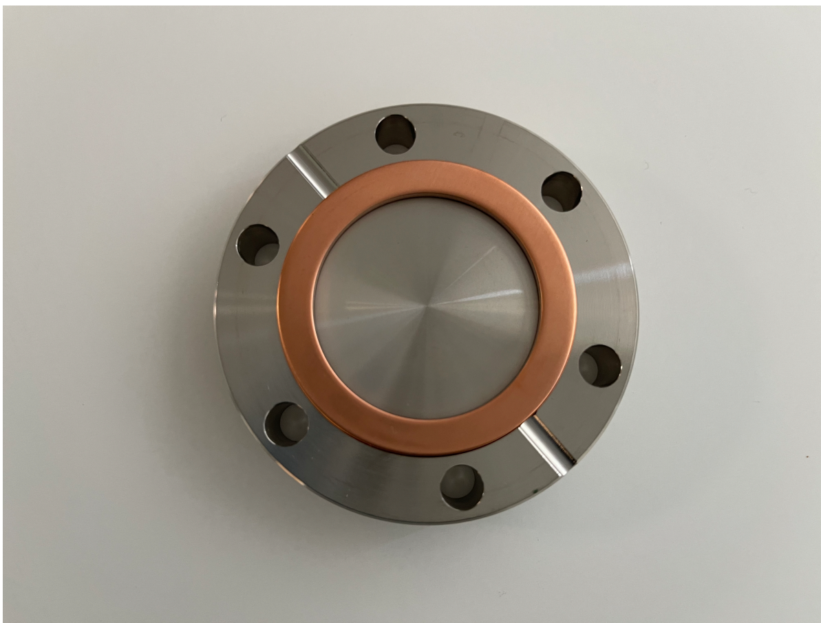
Figure 3.7.b. CF fitting with copper gasket partially assembled. Photo provided by Elena Brewer, SUNY Erie Community College.
