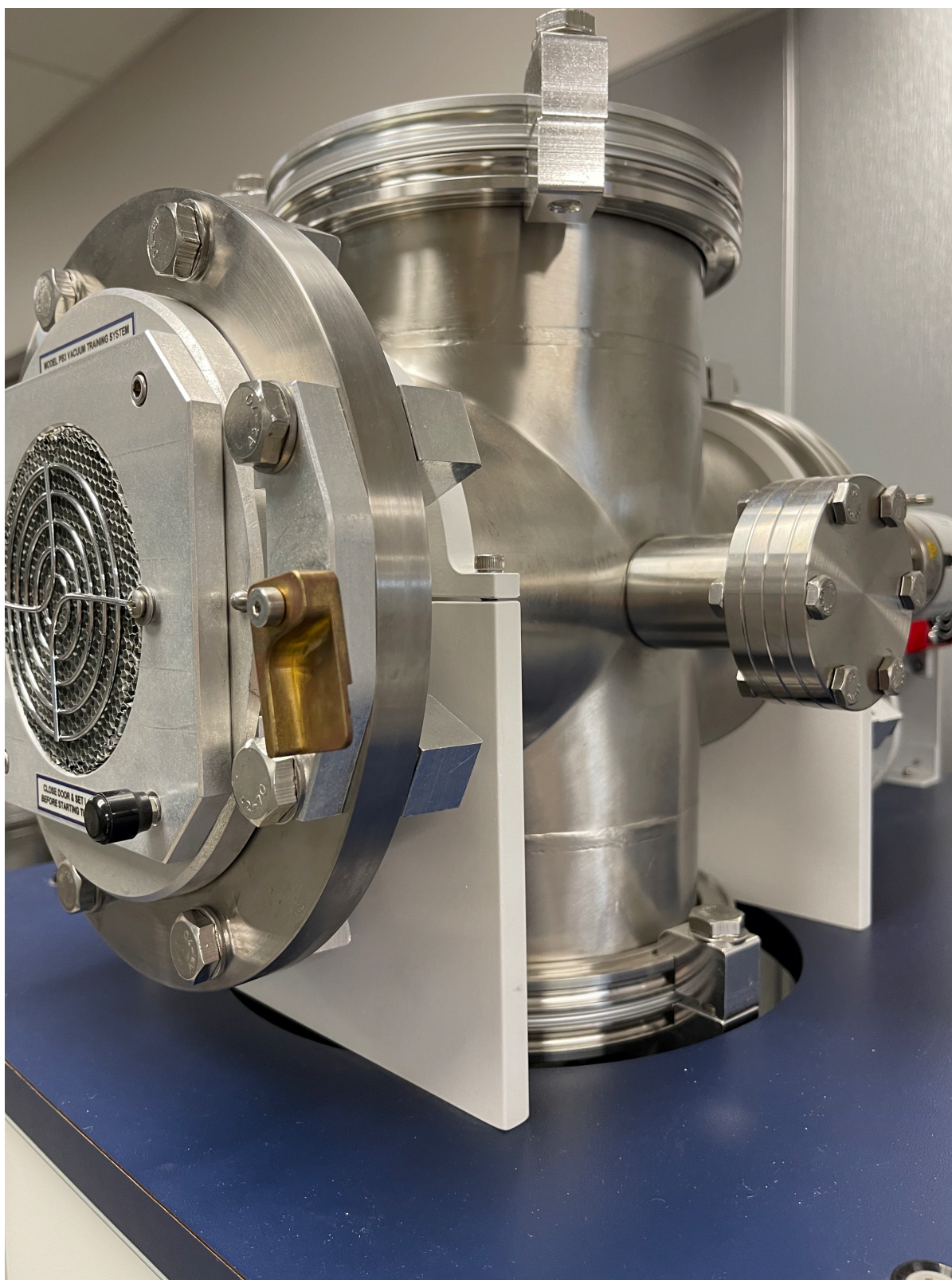
Figure 3.5.a. Stainless-steel chamber. Photo provided by Elena Brewer, SUNY Erie Community College.
