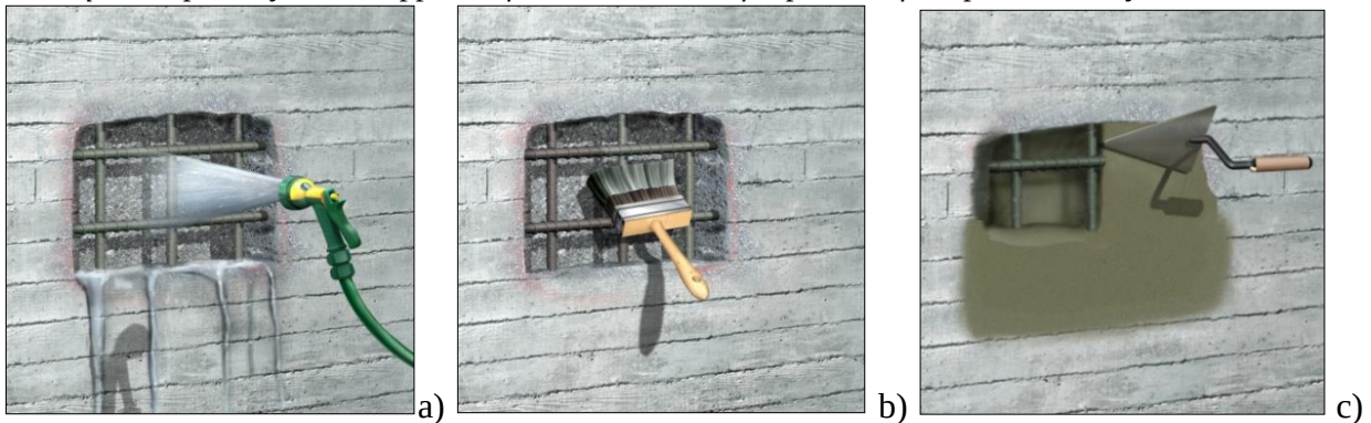
Fig. 2. Sequence of concrete repair.
