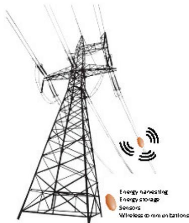
**Figure 1.** Schematic of wireless monitoring of transmission lines.
