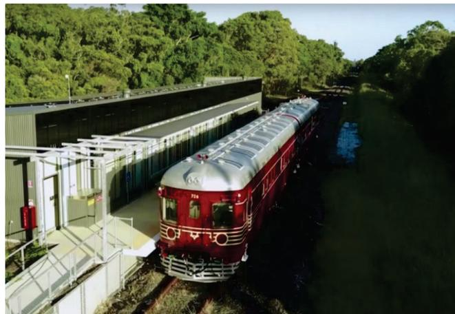
Figure 3. Australia's train with PV solar panels [21].
