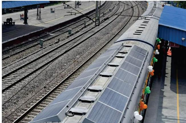
Figure 2. The UNESCO train with PV solar panels [20].
