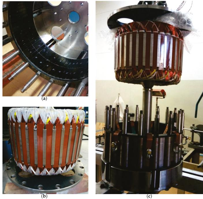
**Figure 24.** Machine construction: (a) all sets of PMs are mounted onto the rotor core, (b) side view of wound stator with distributed overlapping windings, and (c) assembling of the PMVM prototype.
