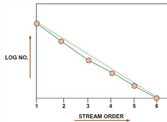
Figure 5-46. Plot of the logarithm of the number of streams of a given order against the stream order, for a given drainage basin.
