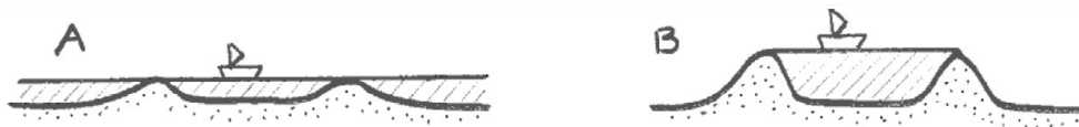
Figure 3-49. The stage of a flood flow for a given flood discharge. A) Before building of levees. B) After building of levees.
