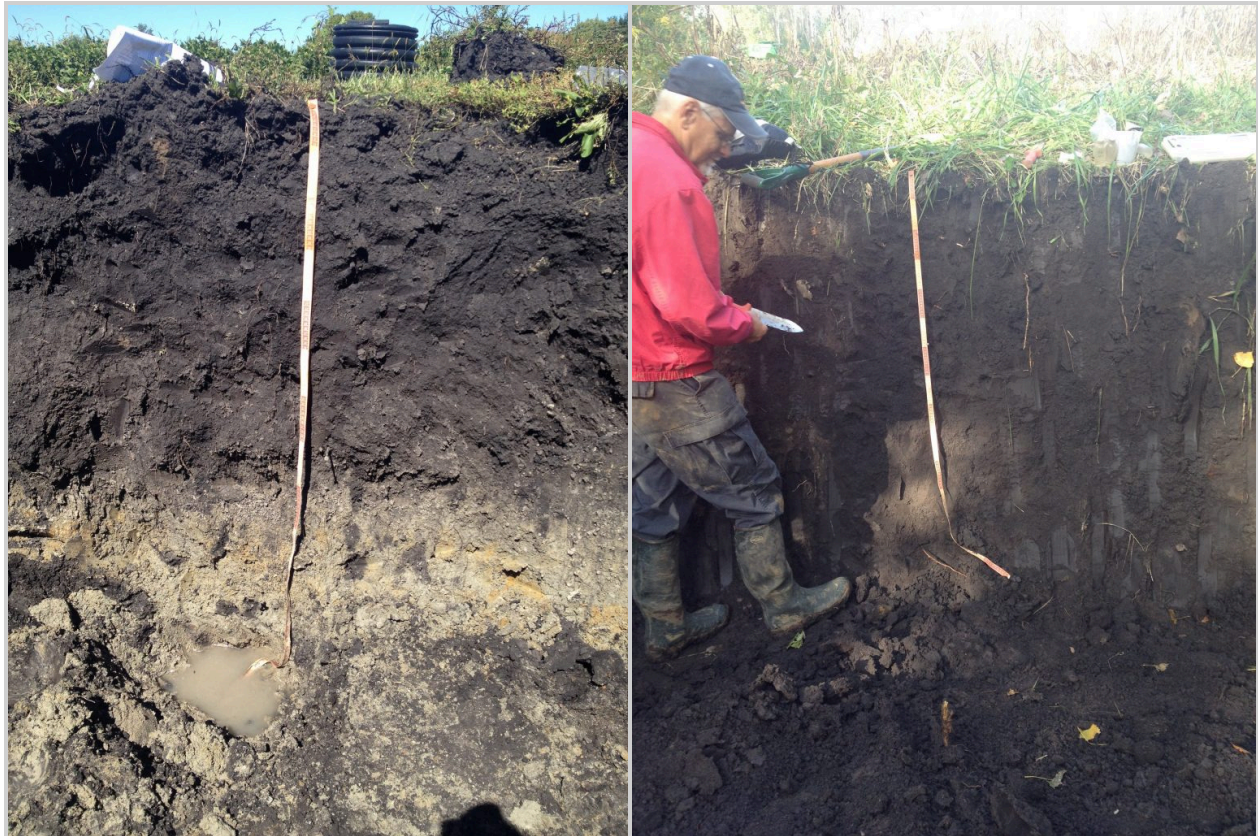
This image and the one to the right show a large accumulation of organic matter in the top horizon. Photo Credit: Amber Anderson.
