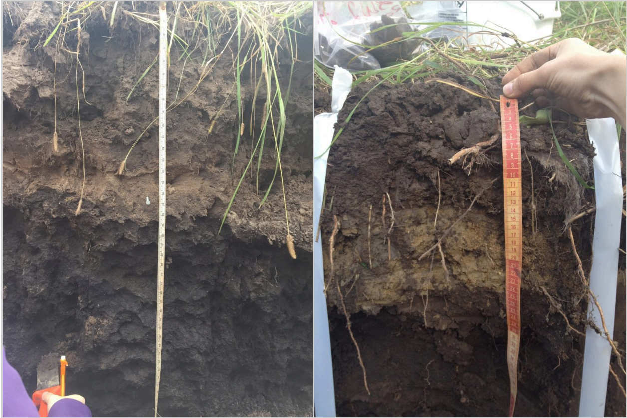
This soil, found on the Kansas river flood plain, shows significant recent deposits burying the prior surface. This soil, found at the base of a hill in Iowa, shows evidence of recent instability uphill, as the surface 25-30 cm are on top of the prior surface. Photo credit: Amber Anderson
