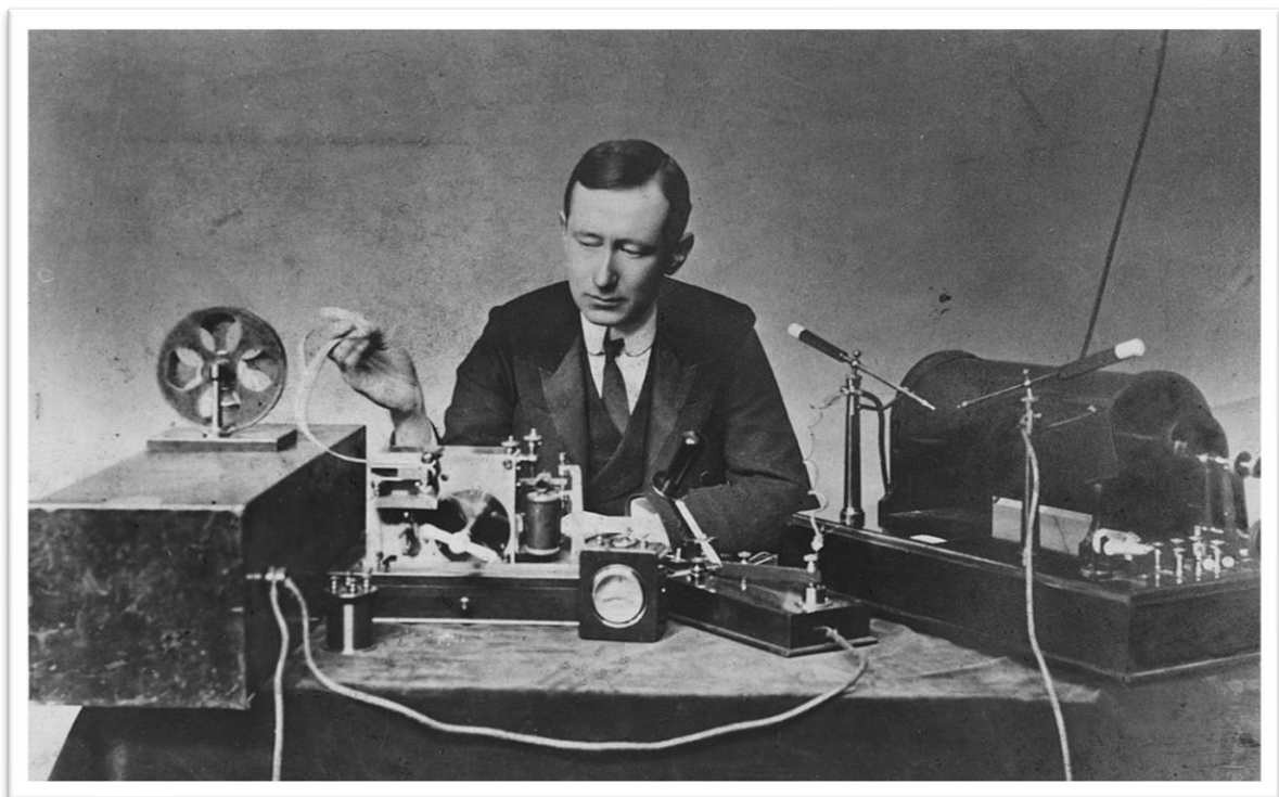
Electrical engineer and inventor Guglielmo Marconi with the spark-gap transmitter (right) and coherer receiver (left) he used in some of his first long-distance radiotelegraphy transmissions during the 1890s.
