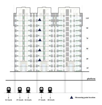
Figure 3. The sectional view of the over-track building.
