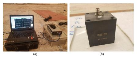
Figure 3. The schematic diagram of the test setup: (a) data acquisition instrument; (b) magnetoelectric vertical acceleration sensor.
