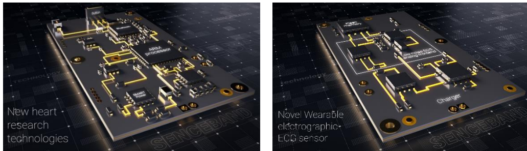
Fig. 1. 3D model of printed circuit board (PCB) of portable ECG-sensor
