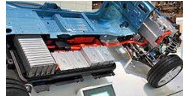
Nissan Leaf's lithium-ion battery pack.
