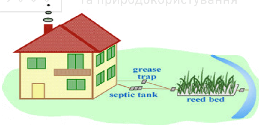
Figure 2. Scheme of constructed wetland iii [3]
