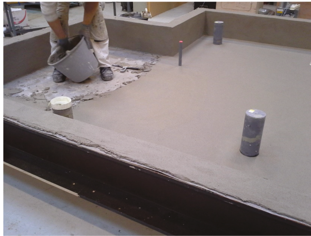
Figure 7. Mounting the test material inside the mock-up for System E, which is a two-component fixed mortar paste combined with edge reinforcements, epoxy and elastic pipe collars.
