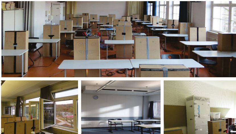
Figure 6. Experimental set up (top), exemplary window ventilation (bottom left), exemplary decentralised ventilation system (bottom middle), exemplary air purifier (bottom right).
