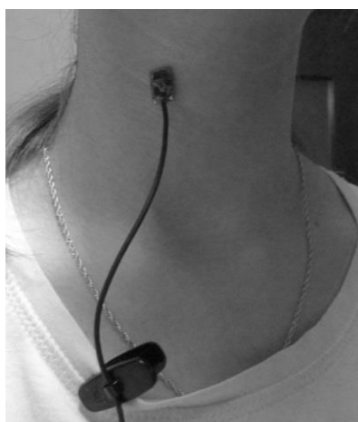
Fig. 2. The sensor mounted on the subjects' neck and measuring acceleration signals Source: private source.
