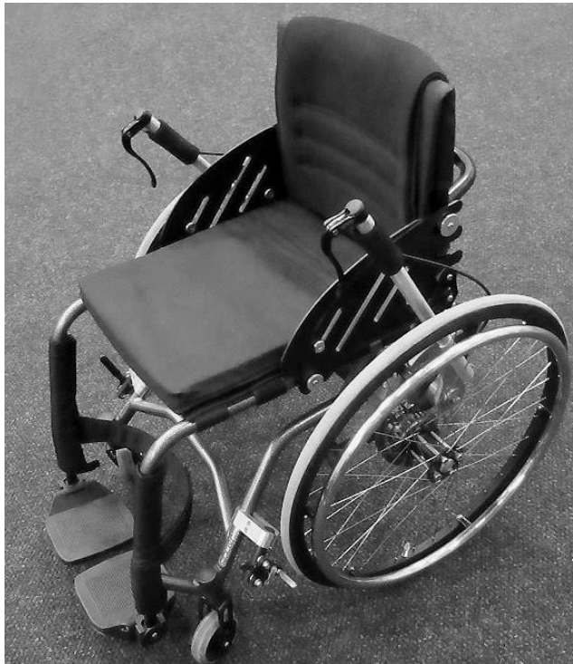
Fig. 1. Wheelchair Prototype DWI1A with lever propulsion mechanism Source: own study.
