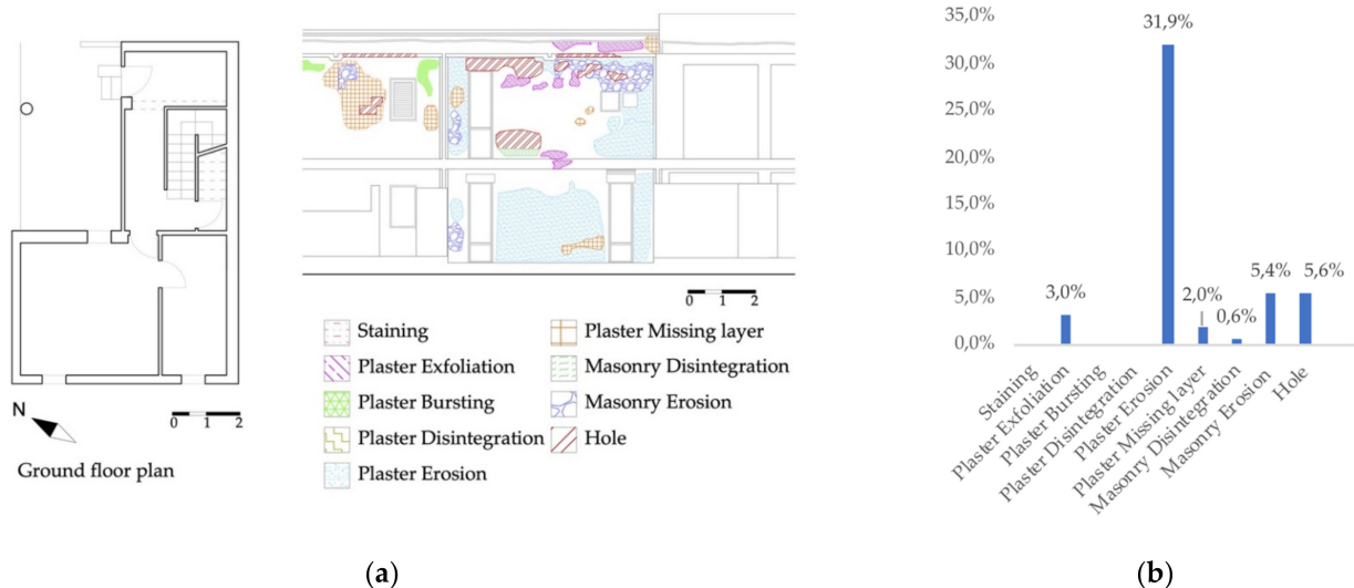
Figure 5. Ground floor plan from Valori project and representation of external visible damages on the façade (a), their extent estimated as a percentage of the analyzed façade surface (b) in the portion A (Figure 4) of the SW elevation of the “L” block. Authors: Erica La Placa, Calogero Vinci.
