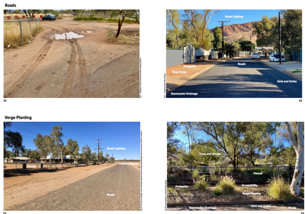
Figure 6. An extract from the Guide to Infrastructure and Housing Standards for Town Camps showing the 'Roads' and 'Verge Planting' topology. The situation found in the Town Camp on the left is contrasted with the same situation typically found outside Town Camps in Alice Springs.
