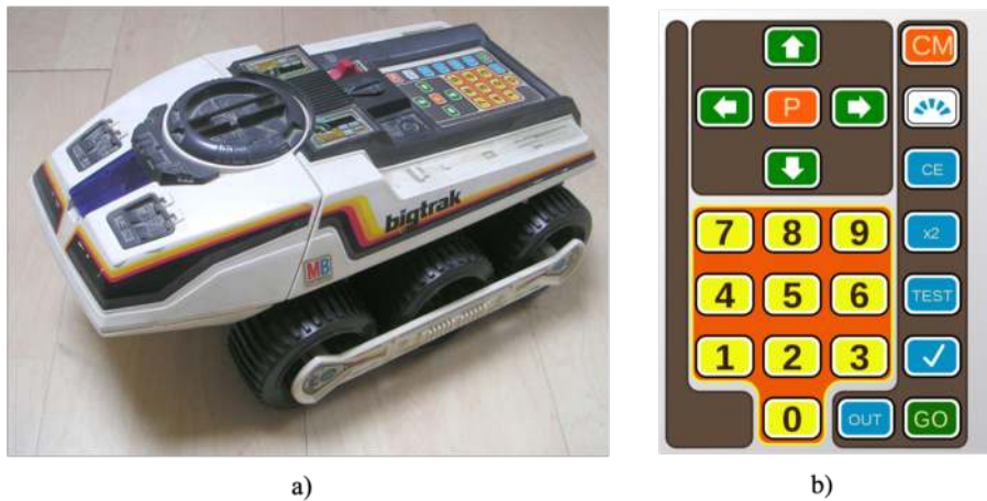
Figure 9.2: (a) Programmable truck BigTrak. (b) Keypad for programming. The keypad shown differs from the one used in the experiment by having a X2 key instead of a RPT key (both figures from WikiMedia Commons, licensed under the terms of the CC-BY-SA-2.0).
